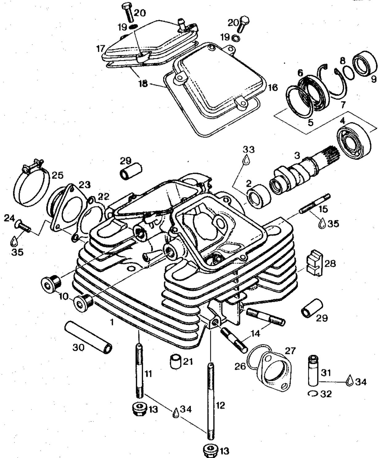
ZYLINDERKOPF, NOCKENWELLE, VENTILDECKEL
